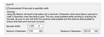
Depending on the barcode type and the values of the connected data source, your results when you use Auto Fit might resemble the following sample labels. Notice that the X dimension of the barcode symbol becomes smaller as the data source (indicated by the human readable text) increases in length so that the symbol maintains its width.
